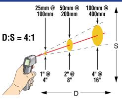
The MiniTempFS is intended for close range, within two feet of the target. The measurement area will be approximately the distance divided by four.
