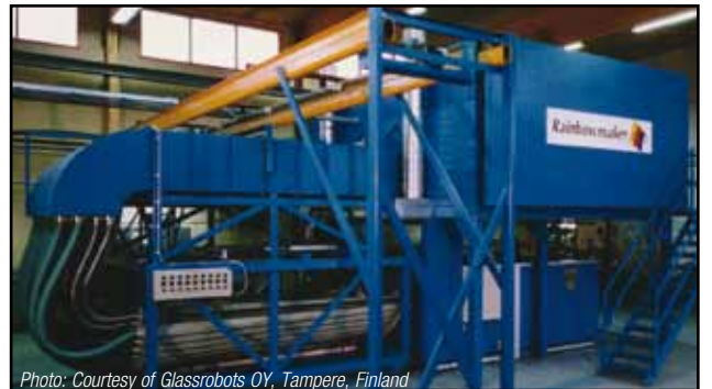
The GS150 System is an automated infrared temperature measurementsystem for glass bending, forming, annealing, and tempering processes.
