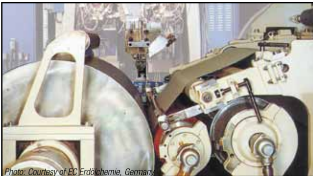
Monitoring edge temperature with EC150 reduces scrap and ensures proper film temperatures for strong film-to-paper adhesion.
